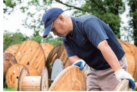
Inspection of collected used drums
