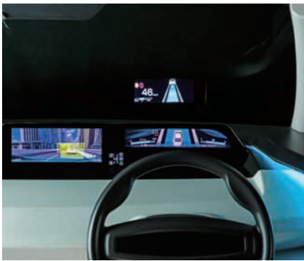
Developing HMIs to convey accurate information to drivers visually and intuitively by combining meters with displays
