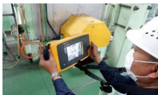
Detecting an air leak location
